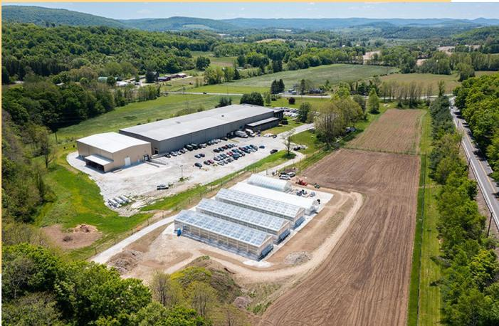
McSweeney designed the layout for a windrow (long, batched piles) composting system that delineated locations for storing feedstocks, pre-composting the wet tea, blending materials, and a pad for the formation and turning of the compost windrows. The design also proposed designated areas to finish, cure, and store the compost product. Further, McSweeney provided guidance on grading, surface preparation, and native plantings that could treat any nutrient-heavy runoff from the compost piles.
