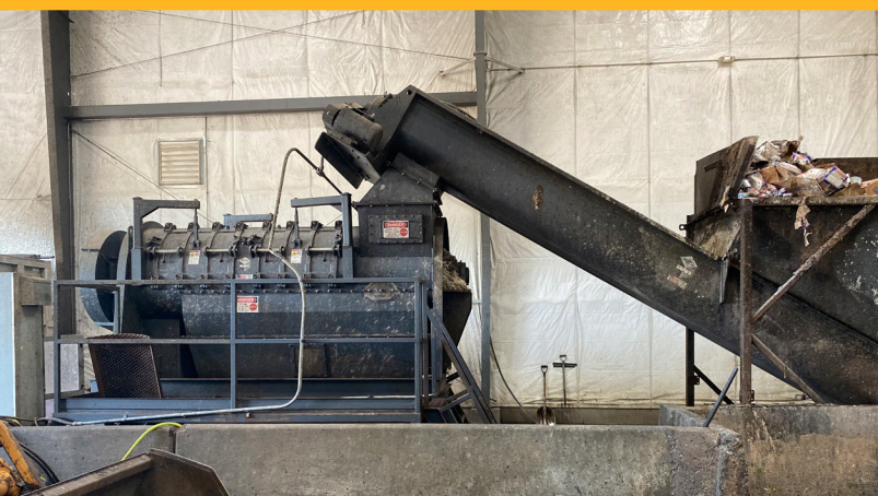
Reinford Farms processes off-spec or out-of-date packaged food in a Scott Equipment Turbo Separator.
