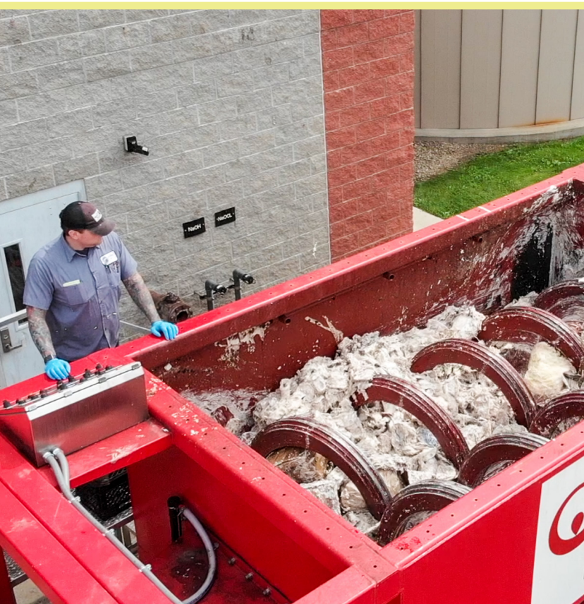
The Hermitage facility's depackager is equipped with a screw press.
