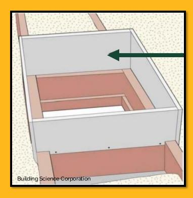
Plywood or OSB as insulation dam
