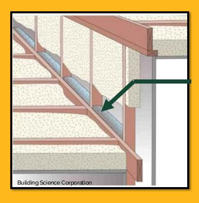
Spray foam covers fiberglass insulation backing.
