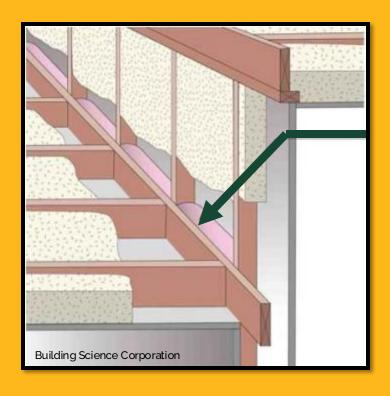
Fiberglass batt insulation as backing for spray foam
