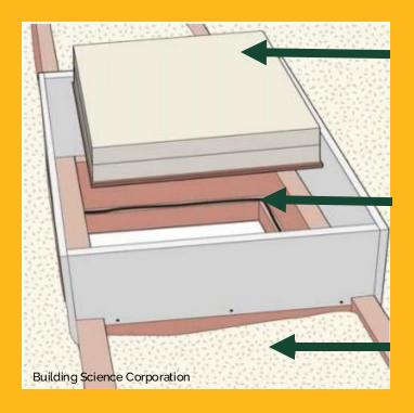
Attach layers of rigid foam board to hatch cover
