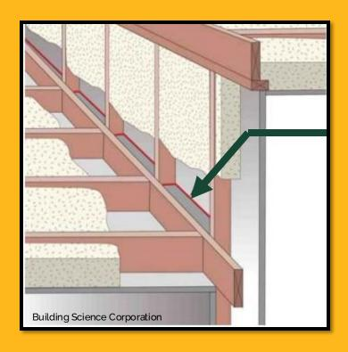
Continuous bead of sealant around entire perimeter of closure
