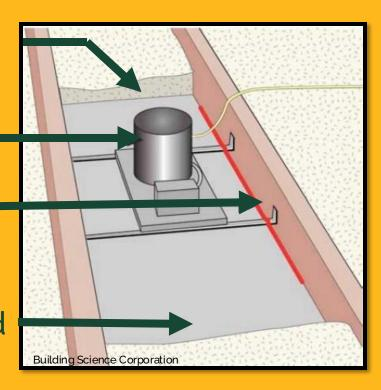
TASK – Control air leakage through the recessed light, control air leakage between the recessed light and gypsum board ceiling, and create an insulation shield.
